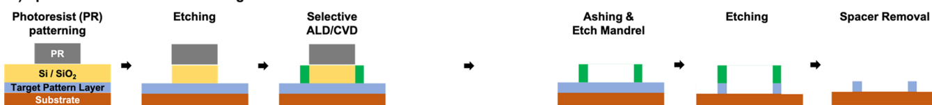
Figure 1. Schematic showing the process for SDDP with (1) conventional ALD/CVD and (2) selective ALD/CVD. Selective oxide deposition enables a reduction in the number of process steps (etch spacer step).
